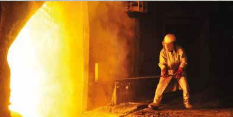
**Running-off of liquid metal melt**
